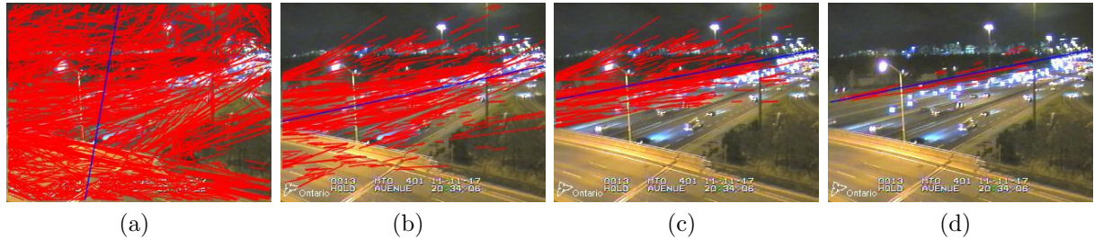
Figure 5.4: Subset of a generated clustering hierarchy tree, showing the accumulated line segments in four nested clusters: (a) root cluster, (b) and (c) two nested clusters with large variance, and (d) a good candidate cluster for a road boundary, which has small variance and a large number of accumulated segments.
