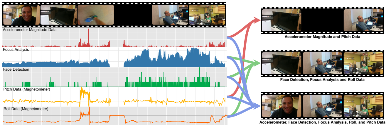
Figure 1. A high-level overview of the capabilities of the proposed system. Frames from the original video, along with time-series plots of both image and sensor data recorded over the course of the video, are shown on the left. The images on the right represent three possible automatically-obtained final-cuts of the same video. These cuts are constructed using different combinations of sensor and visual data streams.
