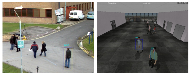
Figure 7: Our visual analysis pipeline is designed from the ground up to work with both synthetic (right) and real video (left) without any modifications. Consequently, our vision pipeline faithfully mimics the performance of a vision pipeline implemented on physical cameras.
